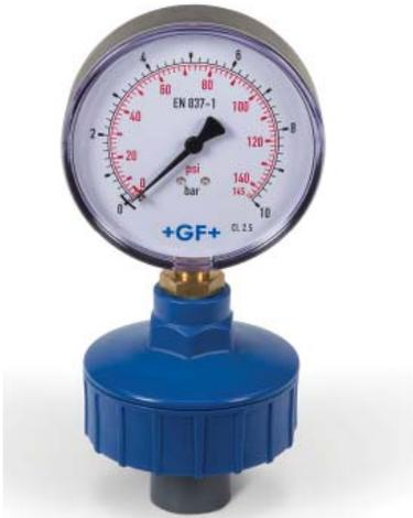
The GF Gauge Guard Type Z500/ Z501 is designed to measure pressure of neutral and aggressive media. The pressure gauge is separated from the medium by a TFM coated EPDM backing diaphragm. Pressure from the pipe/medium side will be transmitted by a buffer fluid.
