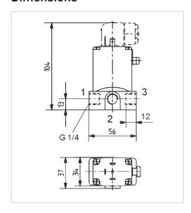
The ports are marked with 1, 2 and 3 as indicated in the configuration table, depending on the circuit function.
