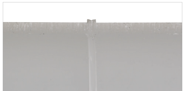
Lateral cut of IR (infrared) welding
